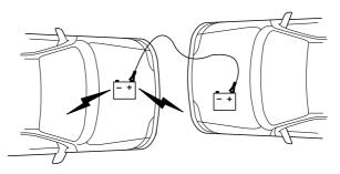
2. Connect the other end of the positive (+) cable to the positive (+) terminal of the assisting battery.
